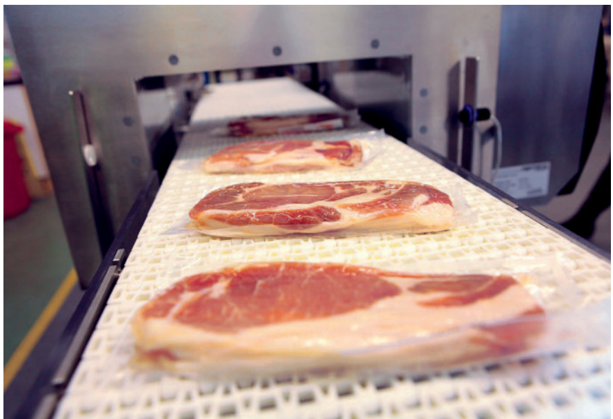
False rejects occur when good product is identified as containing a metal contaminant and can cost a food manufacturer up to £14k annually per line.
