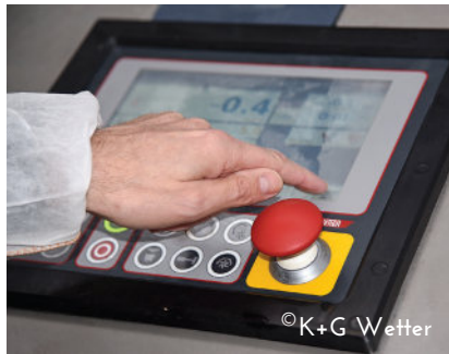
The touch panel, which is integrated as standard into all K+G trade bowl cutters, makes it easy to control the Cutvision and Cutcontrol software solutions.
