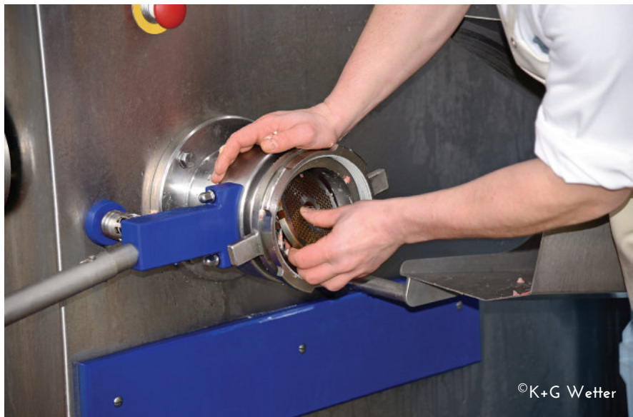
For cleaning, the sorting device can then be dismantled and remounted without the use of tools within seconds.
