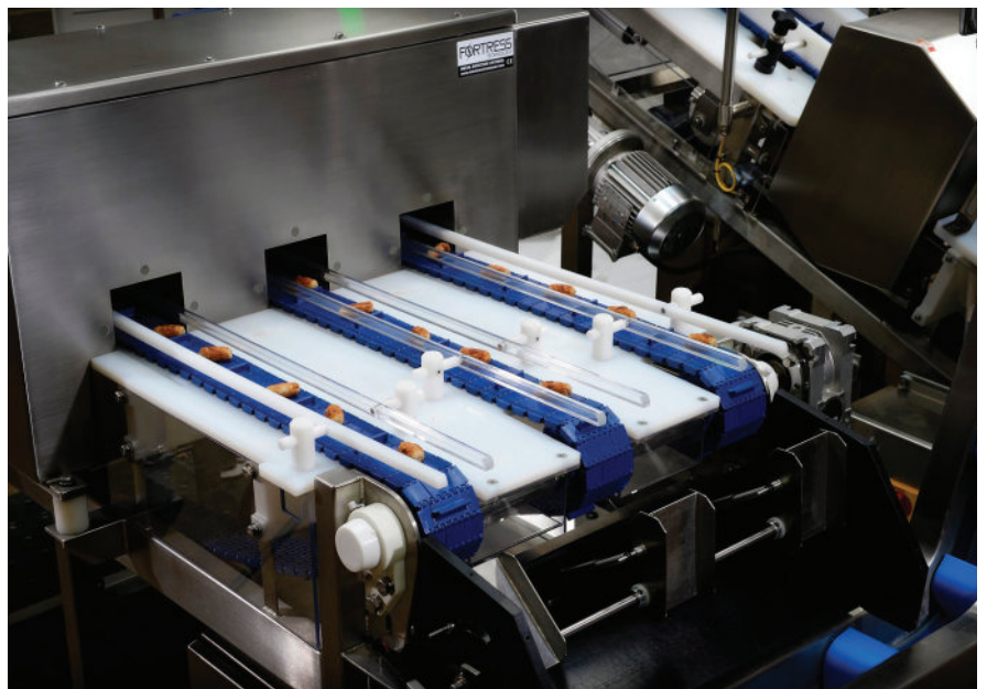
With the multi-aperture, multi-lane metal detector, each lane works independently, enabling a potential contaminant to be isolated without rejecting good product from other lanes.
