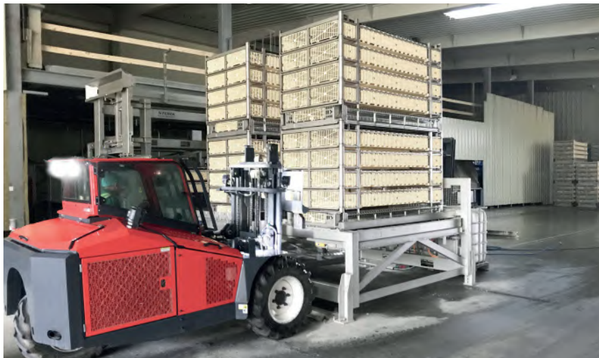
After destacking of the SmartStack modules, birds enter the processing line. Since they left the farm, they have stayed where they are and haven't been touched by humans.
