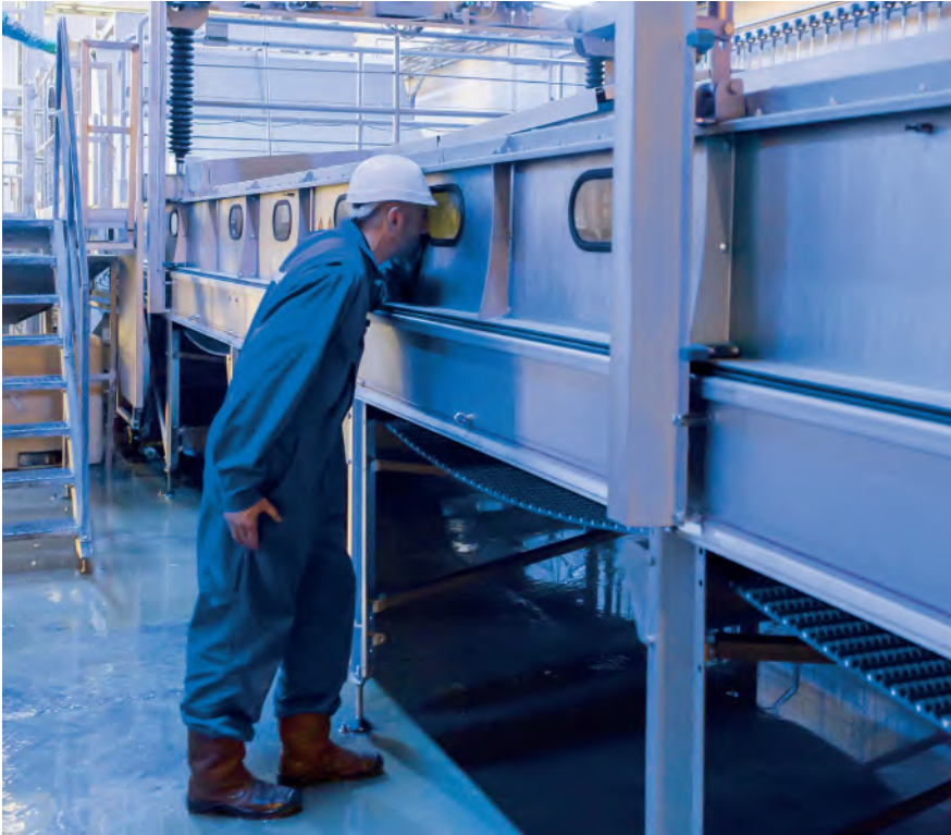
With Controlled Atmosphere Stunning, birds are gradually put to sleep. They no longer experience the stress of being handled and conveyed upside down.
