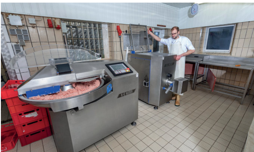
Thanks to the feeder worm, the need to fill the automatic grinder D 114 from K+G Wetter is completely eliminated.
