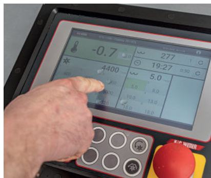
Master butcher Matthias Molitor appreciates the fact that the cutter automatically reduces the RPM when he opens the lid to add seasonings to the sausage meat
