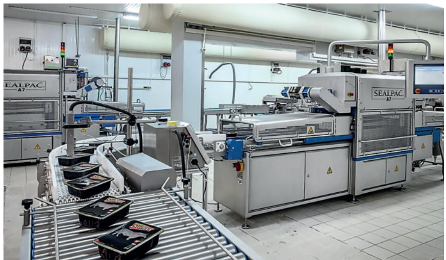
The Sultan Et factory: Two complete line solutions for modified atmosphere packaging of fresh red meat.
