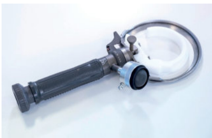
Quantum Flex® trimmers are designed for custom adaptation to the user, by changing the size of the handle, thumb rests and many other exchangeable parts.
