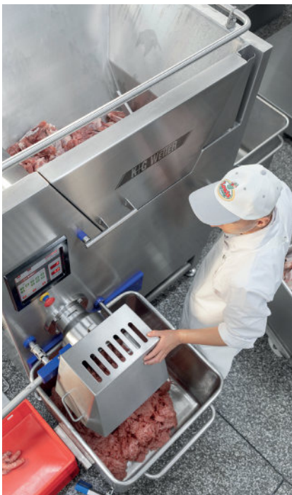
Undesired components such as bone splinters or pieces of sinew are automatically and reliably removed during the grinding process and ejected to the side. Simultaneously, the working area in front of the machine remains free - giving the sorting device of K+G Wetter grinders decisive advantages.
