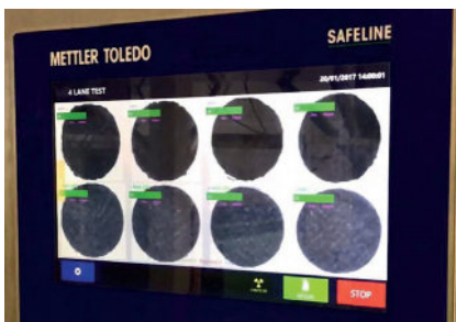
The X39 can inspect and reject non-conforming burger patties in a multi-lane format.
