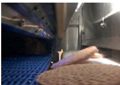
The X39 can inspect and reject non-conforming burger patties in a multi-lane format.
