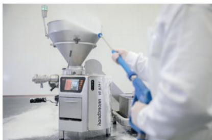
Cleaning with high-pressure cleaner
