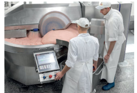
The design of the VCM 360 allows the bowl volume to be utilised optimally – to produce large, top-quality batches without losses caused by overflowing.
