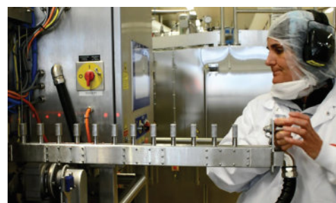
When required, reject confirmation sensors can be pulled out and cleaned, ensuring all products not meeting the pre-defined standards continue to get rejected from production.
