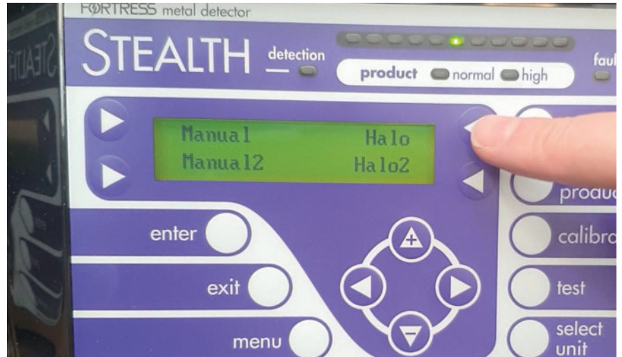
Halo automatically generates a signal calibrated to specified sphere sizes, logging the test results to provide a reliable audit trail
