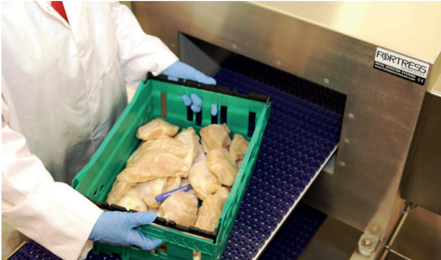
For an accurate test, metal samples should be inserted into the product to ensure it passes through the centerline of the aperture
