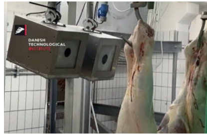
AI Surface Checker detects contaminations on the varying carcass background
