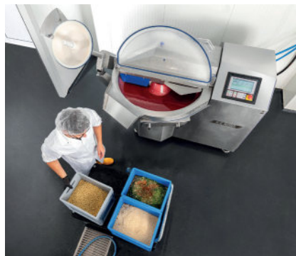
Here, Tressbrüder employee Aurelian-Denis Cocan prepares the mixture for the vegan mini meatballs. The vacuum function of the cutter ensures that the ingredients are perfectly combined.
