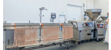
PVLH 251 with pivoting hanging unit and AHE scales
