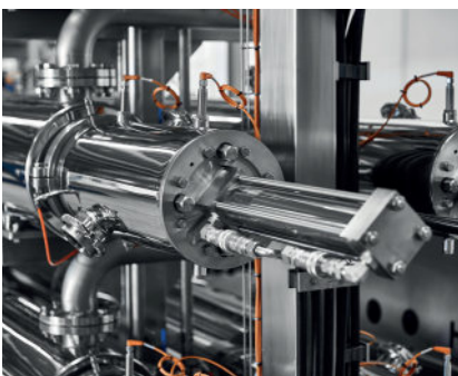
The HRS Unicus Series of reciprocal scraped surface heat exchangers are ideal for cooking and cooling delicate meat products, soups and sauces
