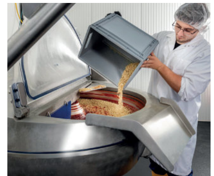
Here, Tressbrüder employee Aurelian-Denis Cocan prepares the mixture for the vegan mini meatballs. The vacuum function of the cutter ensures that the ingredients are perfectly combined.
