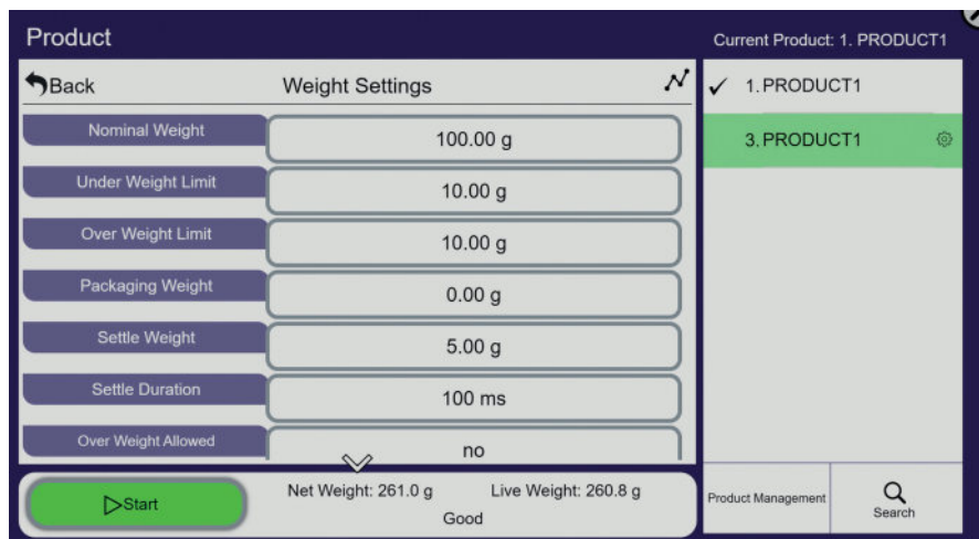
Fortress integrates defined tolerance tables into its Raptor Checkweigher software, providing instant adherence to the local legislative weight regulations.
