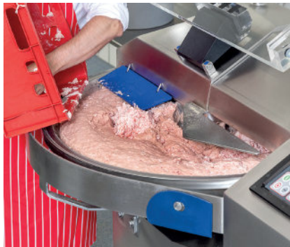
The raised bowl rim on K+G Wetter cutters such as the CM 70 reliably protects against product loss even at maximum filling height.
