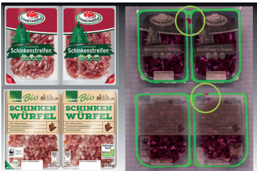
Different packaging variations with seal issues: Notice that HyperScope® is perfectly suited to detect seal issues in the tunnel between two compartments.
