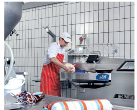
Thanks to the baffle plate, the sausage meat is cut particularly quickly in the reduced cutting chamber, perfectly bound and ready for filling.
