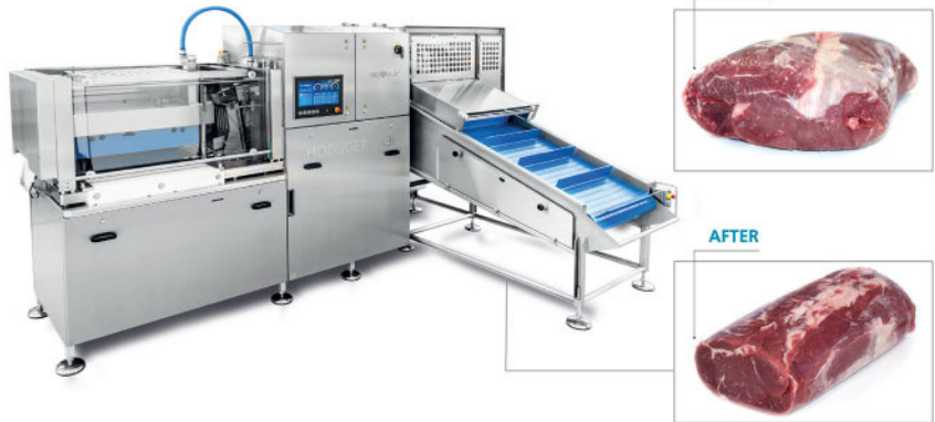
Hoegger® Form Presses: First-class pressing results are achieved even with irregularly shaped products
