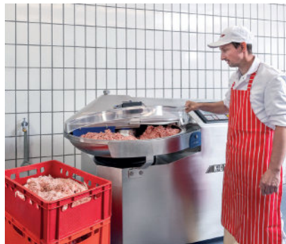
By opening and closing the noise protection lid, Thomas Landes controls the processing steps in the preparation of the basic sausage meat.
