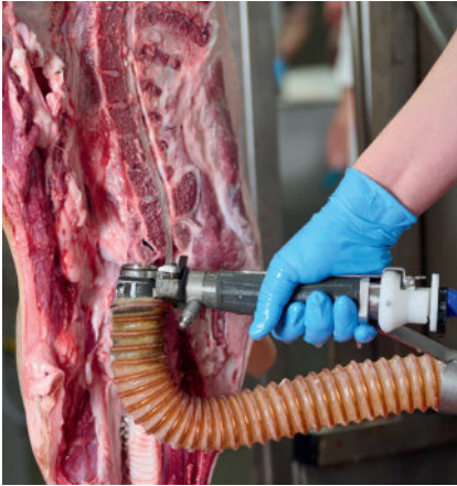
Quantum Flex® TrimVac for the professional and safe removal of potentially hazardous spinal cord tissue
