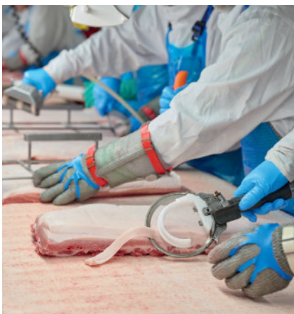
Quantum Flex® Trimmer from Bettcher for clean, trimming of meat without damaging the precious parts
